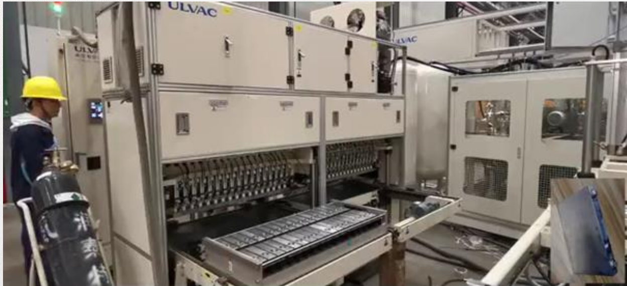
Helium Bombing Leak Testing System for Lithium Battery [Rectangular Power Lithium Battery ]
